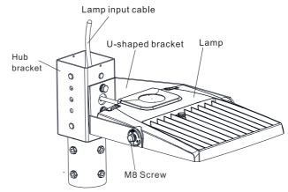
3. Screw the light fixture onto the U-shaped bracket, and thread the cable through the waterproof cover. Fix several other lamps in the same way.
