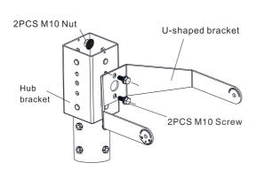
Connect the U-shaped bracket and the convert bracket with screws;
