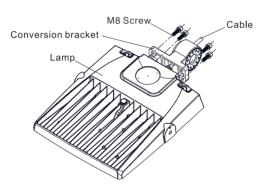
3. The cable passes through the conversion bracket and is fixed conversion bracket to the lamp with M8 screws.
