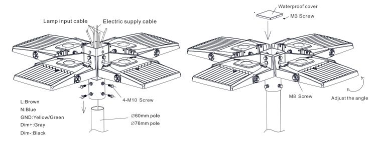
4.Use screws to securely fix the assembled lamp to the lamp pole; Each lamp's cable is connected in parallel with the mains cable and the wire ends are hidden inside the lamp pole.
