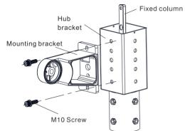
2. Secure bracket D to the hub using screws and nuts;
