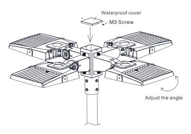
6.Install the waterproof cover onto the top of the adapter bracket and secure it with screws; Adjust the light output angle and fix the lamp to ensure reliable installation.
