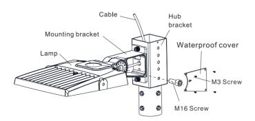
4. Thread the wire through the mounting bracket, fix the lamp to the hub with M16 screws, secure the waterproof cover, and install other lamps in sequence;
